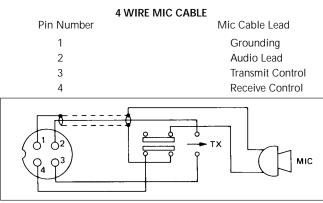
Fig. 1. Cobra 148 GTL ST microphone schematic.
